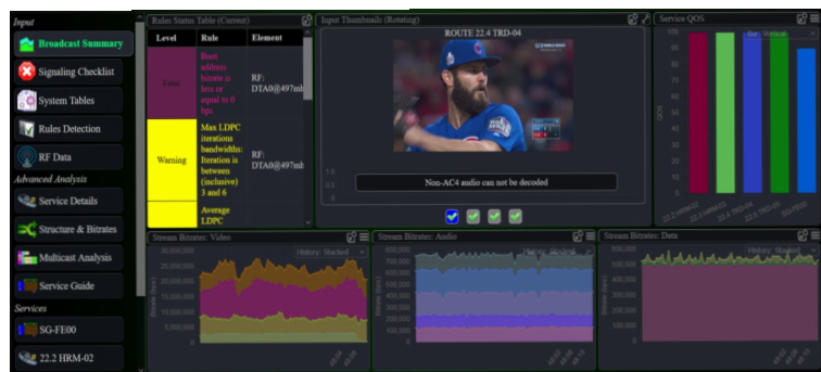
Drill down to real-time details of ATSC 3.0 inputs, services, and elementary streams.
