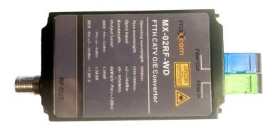
\*Note: This device is compatible with all analog optical transmitters used to transmit analog and digital RF carriers. It is not designed to receive data only signals such as 1gig, 10gig or Ethernet type circuits...
