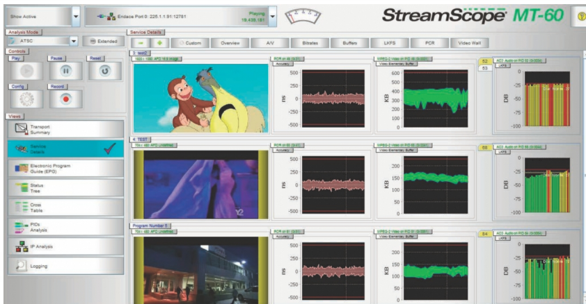
Field-proven ATSC 1.0 MPEG transport stream analysis for Ethernet, RF, ASI, remote monitor, and TP file inputs.
