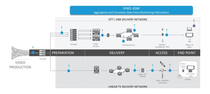
Real-time visualization of service quality drives the focus of operations teams on the most critical events. iVMS ASM is capable of aggregating hundreds of video monitoring points into a single pane of glass so video service providers can easily assess the status of media quality and network delivery.
