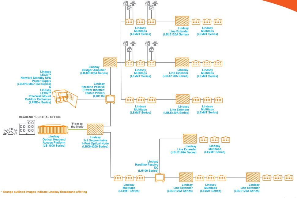
Lindsay combines our LB-1000 optical platform with our LBON4200 2x2 segmentable node to place fiber deeper into the system network. RF output from the optical node feeds the coax architecture, LB-MB-120A bridger amplifiers, and LBLE-100A line extenders through to Lindsay's LExMT series of multitaps to give a complete end-to-end hybrid fiber coax (HFC) architecture.
