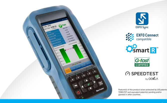
Efficient copper characterization to 35 MHz and DSL/Gfast analysis for the installation and maintenance of ultra-broadband deployments
