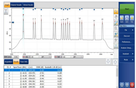
The FTBx-5235 displays channel power, channel wavelength and OSNR. Above: example of CWDM network OSA display. Below: example of DWDM network OSA display.
