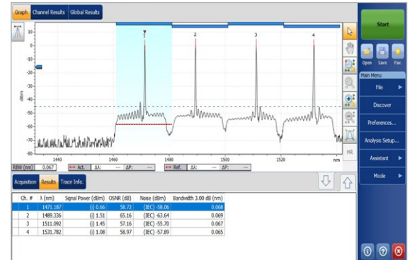
The FTBx-5235 displays channel power, channel wavelength and OSNR. Above: example of CWDM network OSA display. Below: example of DWDM network OSA display.
