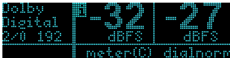
Figure 7: Digital Program Measurement (showing incorrect dialnorm value)
