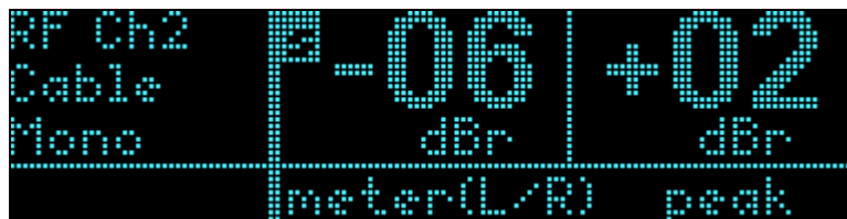
Figure 10: LM100 Display while RF Input is Active (mono channel shown)
