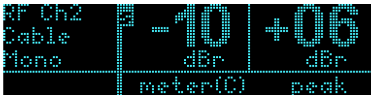
Figure 4: Leq(A) RF Input Dialogue Level Set Incorrectly to -10dBr
