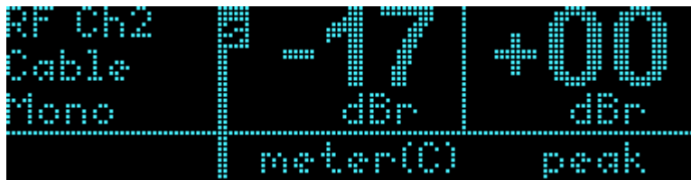
Figure 2: Leq(A) RF Input Dialogue Level Set Correctly at -17dBr
